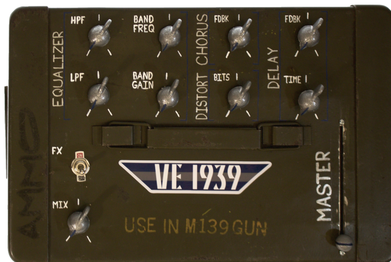
Figure 1: Finished VE1939 box using ammo box and custom knobs to create a retro aesthetic
