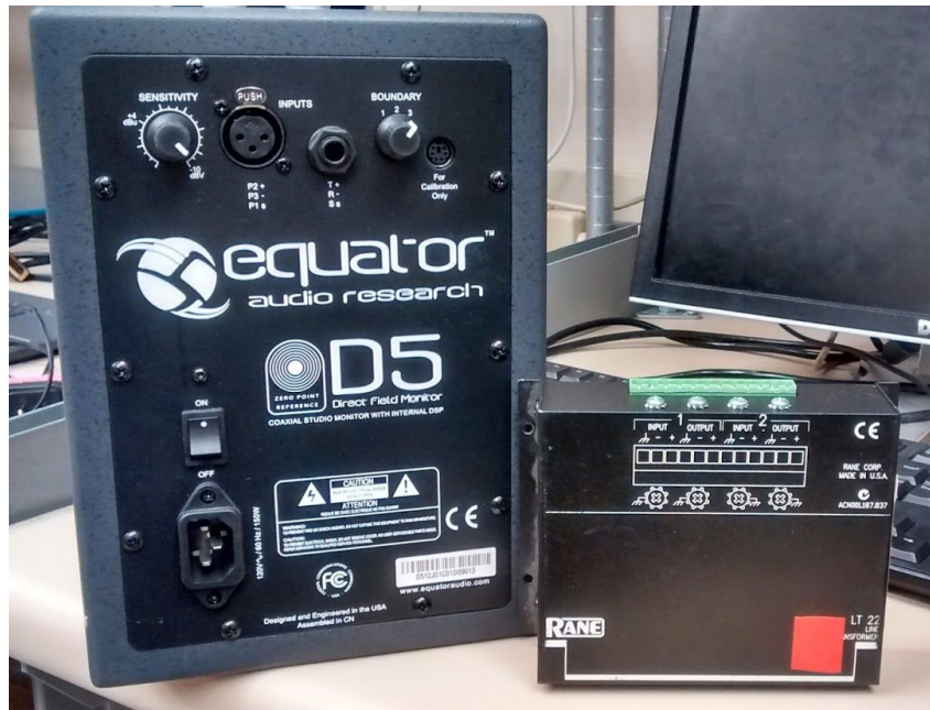
Figure G.4: Speakers and Isolation Transformer
